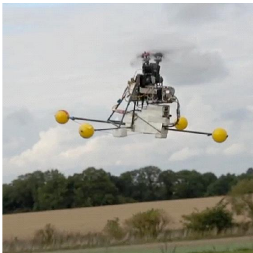
Figure13. Meshing, tilting rotors in helicopter mode flight tests of the 1/20^{\text{th}} scale model
