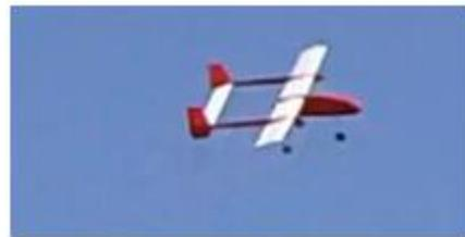
**Figure 16. This shows the airplane mode 1/10<sup>th</sup> scale model, built and flown by Chris Gladwin (Ref. 15).**
