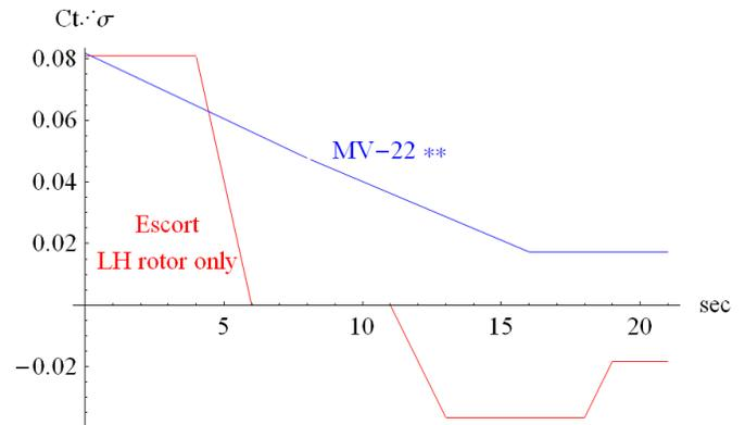
**Figure 9. Proprotor blade loading  $C_t/\sigma$  for the conversion shown in Figure 7 for the Escort (LH rotor shown) and the MV-22 \*\* (author's estimates).**
