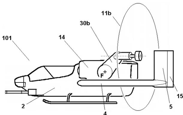
Figure 4. The 6B configuration chosen in Figure 3 is shown here in more detail in airplane mode where the rotors operate as pusher props.
