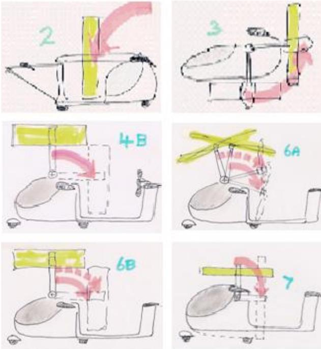
Figure 3. Six cartoons of some centre-line tiltrotor configurations showing transition from helicopter to airplane mode. A single solid arrow indicates that both rotors transition together. Two arrows, solid and dotted, show rotors that transition is one-at-a-time. 6B was the final selection.
