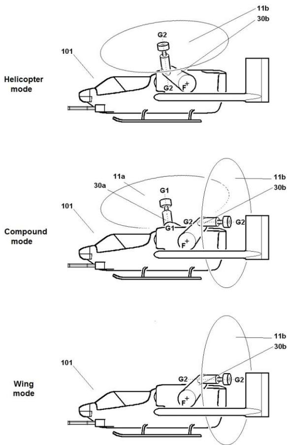
**Figure 6.** Within the conversion corridor, the rotors can be tilted one-at-a-time between the helicopter and wing modes. The transitioning rotor's thrust is kept substantially zero, while the other rotor maintains the flight thrust.
