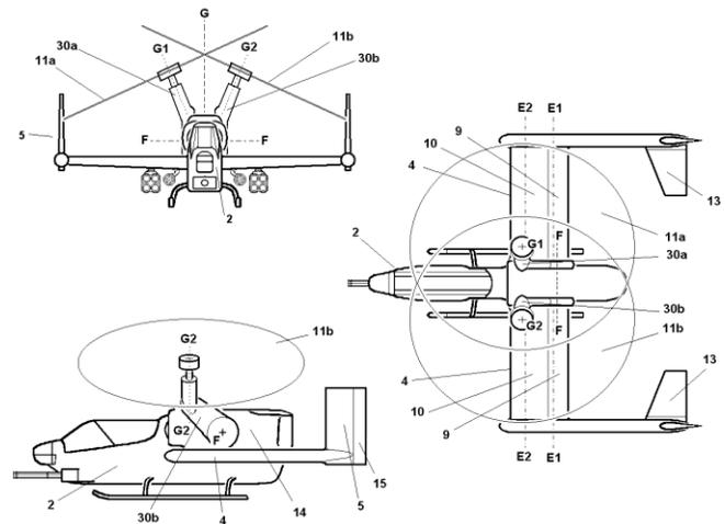
**Figure 5. Three views of the Escort in the hover mode. The meshing rotors are tiltable about the F-F axis.**
