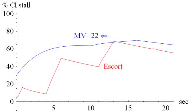
**Figure 8. Wing coefficients of lift  $C_l$ , as a % of stall, during the transitions shown in Figure 7 for the Escort and the MV-22 \*\* (author's estimates).**
