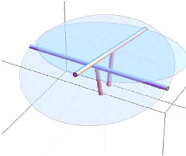
**Figure 13. Snapshot from 3D animated math model of blade meshing. Rotors canted  $11^\circ$  to the XZ plane and tilted to  $90^\circ$  vertical. Axis of tilt offset vertically towards the rotor hubs. Projected area is 1.3 times a single disk.**
