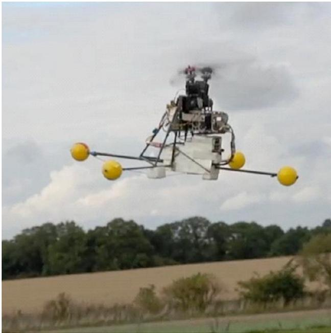
**Figure14. Meshing, tilting rotors in helicopter mode flight tests of the 1/20<sup>th</sup> scale model**
