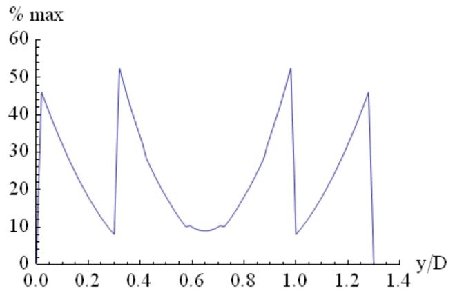
**Figure 18. Local disk loading as a % of maximum; y is the lateral distance, left to right, through the rotor hubs; D the diameter of an individual disk. The plot is for disks that overlap by 0.3 D between hubs.**
