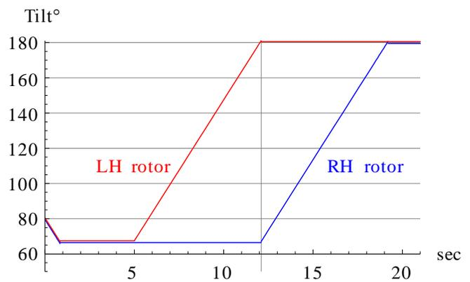
**Figure 10. Piecewise one-at-a-time tilting as used in the math model for the conversion of Figure 7.**
