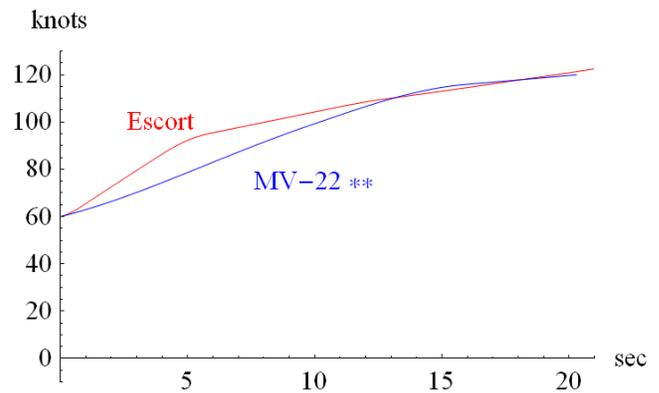
**Figure 7.** The Escort and the MV-22 \*\* (author's estimates) transitioning from 60 knots in helicopter mode to about 115 knots in airplane mode.
