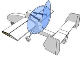
**Figure 19. This is a suggestion for a single boom configuration for the 1/10<sup>th</sup> scale model flight tests.**
