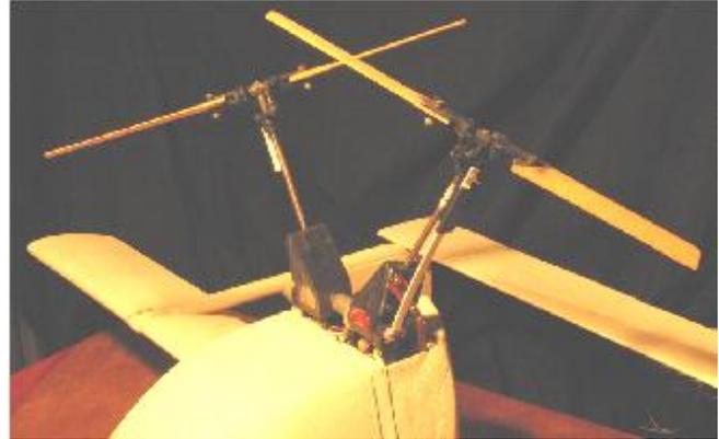
**Figure 11. Mechanical model used to demonstrate one-at-a-time tilting of intermeshing rotors to a pusher prop position.**
